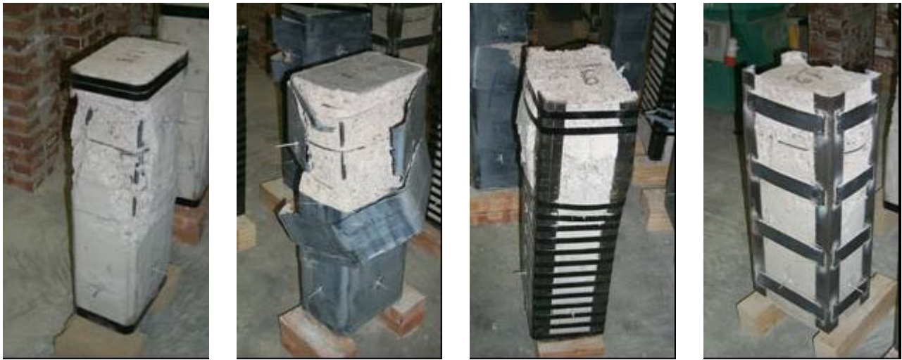
Fig. 6: Typical failures observed in the reinforced columns
